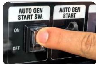
3. When the AUTO GEN START connected, the external intelligent control system controls the start and stop of the generator (it will start and run if the two wires are Short-circuited, and shut down if they are disconnected).
