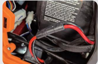
**Note:** The generator is equipped with a battery charging feature. Once the engine is running, a small current will slowly recharge the battery.
