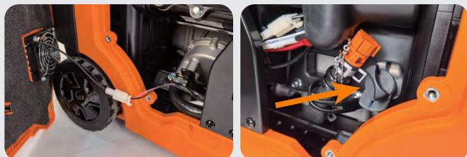
3. Using a funnel, as needed, add the appropriate type of oil until the oil level is at the proper level.
