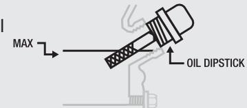
5. After refueling, tighten the oil dipstick, wipe off the surrounding oil.
