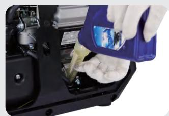
5. After refueling, tighten the dipstick and wipe off the surrounding oil stains.
