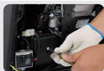
3. Remove the air filter element.
