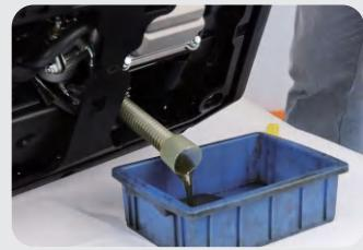
4. Follow the procedure of "Adding Engine Oil" to add new engine oil and check the oil level.
