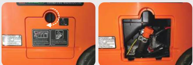
3. Place an oil pan under the engine, tilt the generator to quickly pour out oil;
