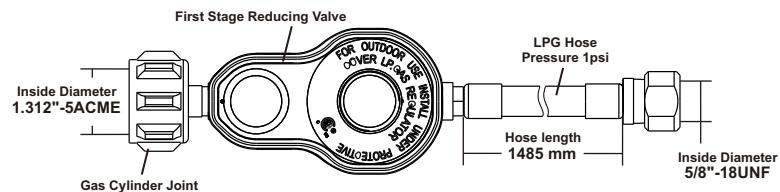
Connect the LPG tank to transmit LPG fuel to the generator.
