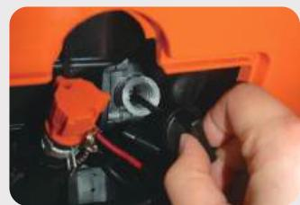
5. Refill oil to a proper level, tighten oil dipstick, cover external cover plate and tighten the knob.
