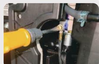
6. Allow fuel to drain into the container and tighten the drain screws on the carburetor. Install the engine service panel.
