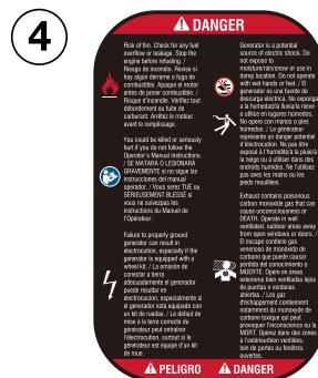
Before using the generator, please read the operation manual. Be careful with the shock hazard. Be careful, the fuel is flammable, do not add the fuel when the engine is running.
