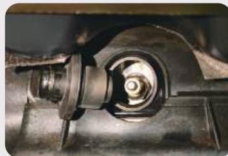
2. Insert the screwdriver into the sleeve, to screw it counterclockwise, and then remove the spark plug;
