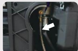
5. Loosen the carburetor drain screws until you see fuel draining from the carburetor.
