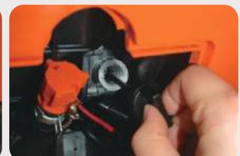
3. Fill in 0.18gal(0.7L) oil (SAE 10W/30 oil is recommended, of which the grade is API standard Type SE or higher);
