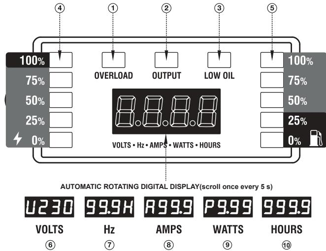
① **OVERLOAD:** Red light means the machine overload.
