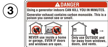
Do not use the generator in door or garage, the exhaust contains carbon monoxide, this is a poison you cannot see or smell, and it will kill you in minutes.
