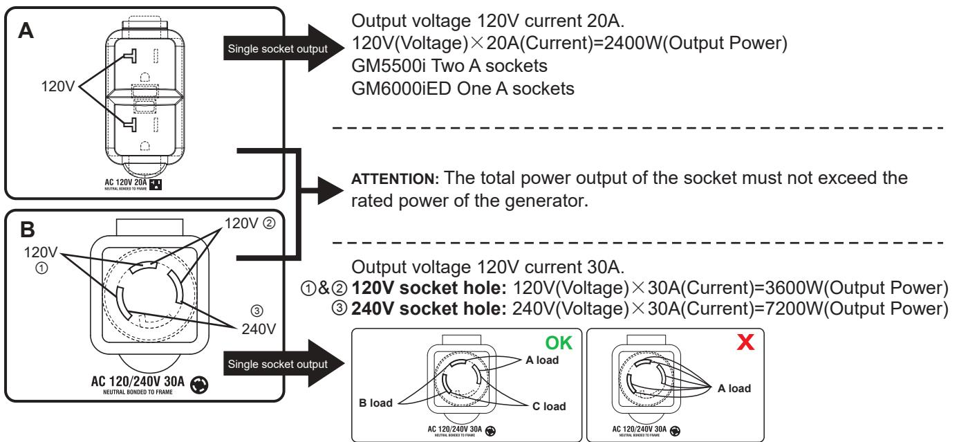
**ATTENTION:** ①②③ can output at the same time, but the total power output of the socket can not exceed the rated power of the generator, can not be connected to the same load.
