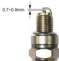
**Tip:** The spark plug clearance is required to be measured by line thickness gauge, which shall be adjusted if necessary.
