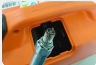
3. Check whether there is discoloration, and remove carbon deposits. Check whether there is little pale to moderate brown on ceramic cores around center electrode of the spark plug;
