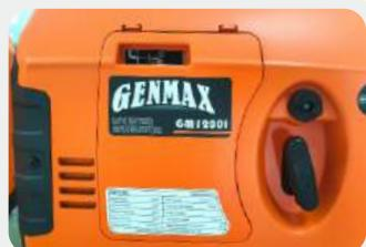
2. Remove screws , to remove cover plate of air cleaner ;
