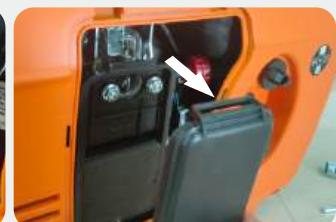
3. Clean foam cleaner element with cleaning solvent and blow it dry, Put a few drops of oil on the filter element.
