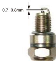
**Tip:** The spark plug clearance is required to be measured by line thickness gauge, which shall be adjusted if necessary.
