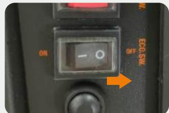
5. Press Engine Switch to "ON";
