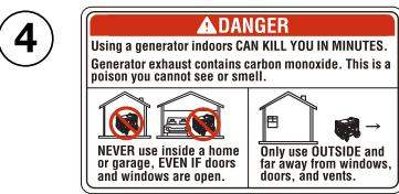
Do not use the generator in door or garage, the exhaust contains carbon monoxide, this is a poison you cannot see or smell, and it will kill you in minutes.
