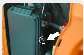
6. Allow fuel to drain into the container and tighten the drain screws on the carburetor. Install the engine service panel.
