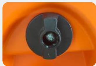
**4.** After the generator has completely cooled down, turn ventilation knob on fuel tank cap to "OFF".
