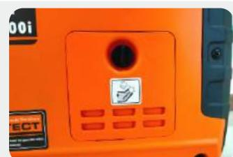
3. Unscrew oil dipstick, Fill in 0.09gal(0.33L) oil (SAE 10W/30 oil is recommended, of which the grade is API standard Type SE or higher);
