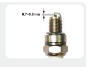
Tip: The spark plug clearance is required to be measured by line thickness gauge, which shall be adjusted if necessary.
