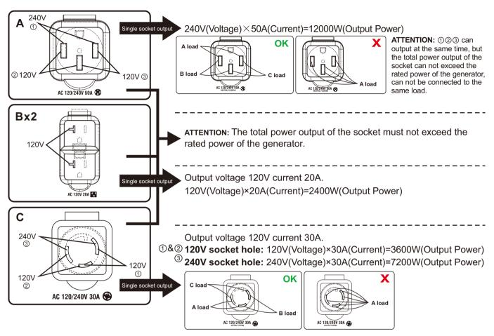
**ATTENTION:** ①②③ can output at the same time, but the total power output of the socket can not exceed the rated power of the generator, can not be connected to the same load.
