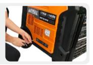
**2.** Connect the positive and negative electrodes of the battery. A quick-connect battery plug is pre-installed on the battery. Remove the cable tie securing the plugs, align colors, then push firmly to connect them.
