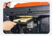
3. Use a soft bristled brush (brush along its folds) or compressed air to remove dust and dirt adhering to the surface of the paper filter element.
