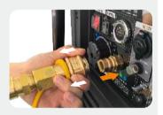
6. Turn the natural gas (NG) supply line valve to the fully open position. Check all connections for leaks by wetting the fittings with a solution of soap and water. Bubbles which appear or bubbles which grow indicate that a leak exists. If a leak exists at a fitting, turn the natural gas (NG) supply line valve to the fully closed position and tighten the fitting. Open the natural gas (NG) supply line valve and recheck the fitting with the soap and water solution.
