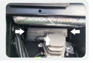
2. Remove the air filter element.
