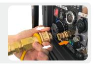
5. Remove the safety plug or cap from the LPG tank valve and attach the other end of the hose to the LPG connector on the tank. Hand-tighten.
