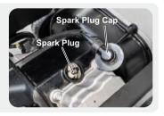
6. Unscrew the spark plug from the generator using the spark plug wrench included with this product.
