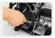
2. Remove the air filter element.
