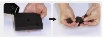
5. Return the air filter element to its original position. Reinstall the air filter cover.
