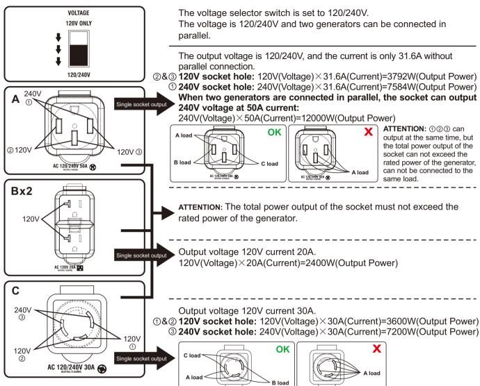
**ATTENTION:** ①②③ can output at the same time, but the total power output of the socket can not exceed the rated power of the generator, can not be connected to the same load.
