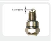
Tip: The spark plug clearance is required to be measured by line thickness gauge, which shall be adjusted if necessary.
