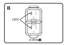
Output voltage 120V current 20A. 120V(Voltage)×20A(Current)=2400W(Output Power)
