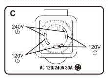
**ATTENTION:** ①②③ can output at the same time, but the total power output of the socket can not exceed the rated power of the generator, can not be connected to the same load.
