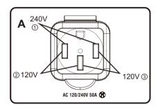
**ATTENTION:** ①②③ can output at the same time, but the total power output of the socket can not exceed the rated power of the generator, can not be connected to the same load.
