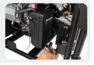
2. Remove the air filter element.
