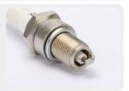
**4.** Check the model of spark plug and clearance.
