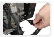
**3.** Place an oil pan (or suitable container) under the oil drain bolt, remove the oil drain bolt and allow the oil to drain;
