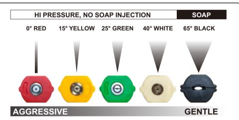
**0° Nozzle-Red:** This nozzle delivers a pinpoint stream of pressurized water and is extremely powerful. Use it for the toughest cleaning jobs, although It covers only a small area. This nozzle should only be directed at surfaces that can withstand intense high pressure such as metal or concrete. Do not use this nozzle to clean wood or soft surfaces.
