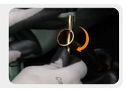
*Tip:* If there is no torque wrench when installing the spark plug, a better estimation method is to screw it 1/4-1/2 turns by force after screwing it in place, but the spark plug shall be screwed to specified torque as soon as possible.
