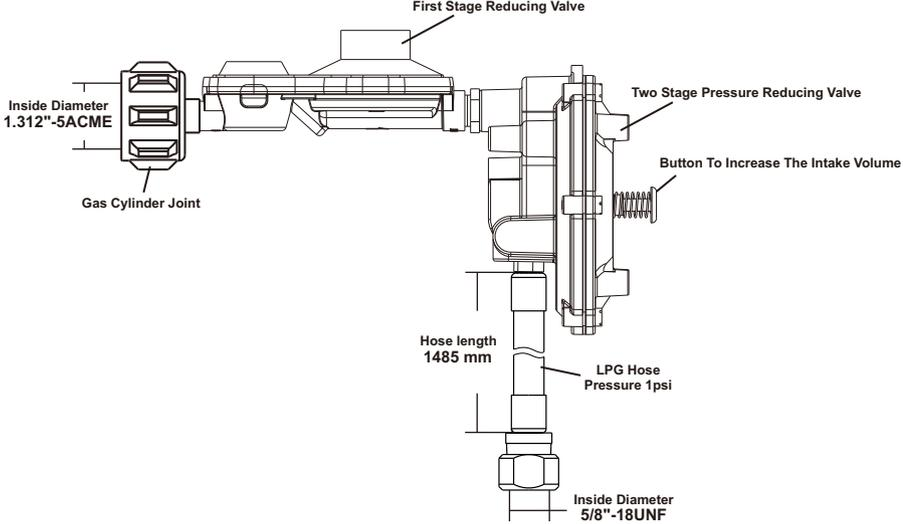
Diagram labels: Inside Diameter 1.312"-5ACME, Gas Cylinder Joint, First Stage Reducing Valve, Two Stage Pressure Reducing Valve, Button To Increase The Intake Volume, Hose length 1485 mm, LPG Hose Pressure 1psi, Inside Diameter 5/8"-18UNF
