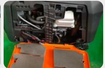
3. Unscrew oil dipstick, Fill in 0.12gal(0.45L) oil (SAE 10W/30 oil is recommended, of which the grade is API standard Type SE or higher);
