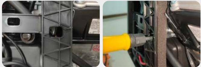
6. Allow fuel to drain into the container and tighten the drain screws on the carburetor. Install the engine service panel.
