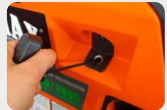
6. After the generator starts, turn the Multi-Switch to "RUN";
