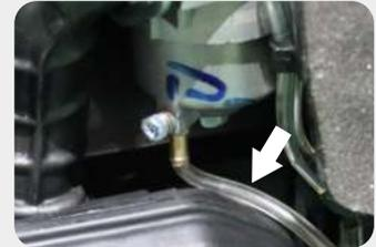
5. Loosen the carburetor drain screws until you see fuel draining from the carburetor.
