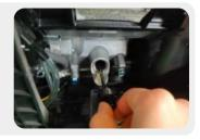
**4.** Place an oil pan under the engine, tilt the generator to quickly pour out oil; After discharging the oil, put the generator back on level ground.
