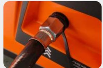
5. Turn the LPG tank valve to the fully open position. Check all connections for leaks by wetting the fittings with a solution of soap and water. Bubbles which appear or bubbles which grow indicate that a leak exists. If a leak exists at a fitting, turn the LPG tank valve to the fully closed position and tighten the fitting. Open the LPG tank valve and recheck the fitting with the soap and water solution. If the leak continues or if the leak is not at a fitting then **DO NOT** use the generator.
