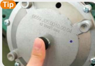
**4.** Press the LOW IDLE Switch to "OFF";
