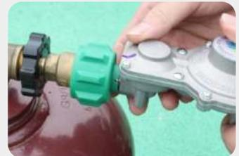
4. Tighten the other end of the LPG hose to the generator intake. Tighten the LPG hose connector with an adjustable wrench until it is snug. **DO NOT** overtighten.
