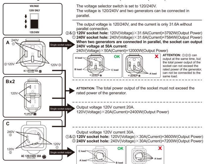
**ATTENTION:** ①②③ can output at the same time, but the total power output of the socket can not exceed the rated power of the generator, can not be connected to the same load.
