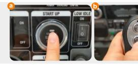
**3.** Press the Main Switch to "OFF"; If not used for more than 48 hours, please turn off the Main Switch.
