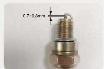
**Tip:** The spark plug clearance is required to be measured by line thickness gauge, which shall be adjusted if necessary.
