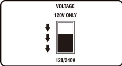
The voltage selector switch is set to 120/240V.
