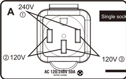
**When two generators are connected in parallel, the socket can output 240V voltage at 50A current:**
