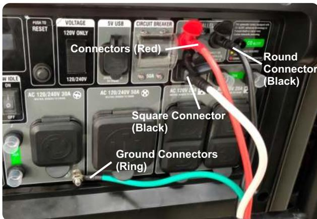
**NOTICE:** If high electrical loads are connected, turn the Low idle switch to the OFF position to reduce voltage changes. With the generators running, make sure both green output indicator lights are ON. If not ON, turn the generators off, restart the generators, and make sure both green output lights are ON.
