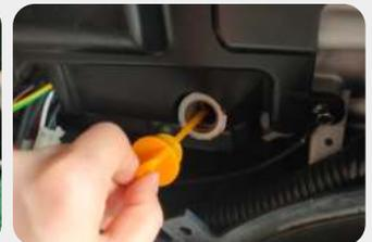
3. Fill in 0.3gal(1L) oil (SAE 10W/30 oil is recommended, of which the grade is API standard Type SE or higher);
