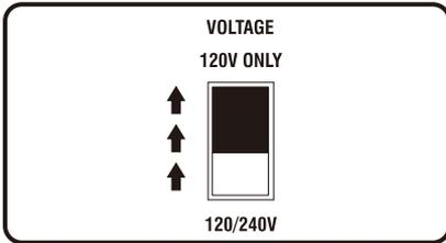
The voltage selector switch is set to 120V ONLY.
