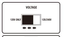
The voltage selector switch is set to 120V ONLY.
