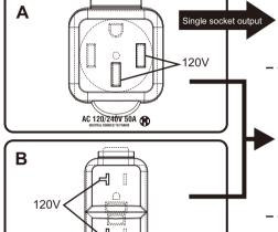
Output voltage can only be 120V and current 50A. 120V(Voltage)×50A(Current)=6000W(Output Power)
