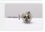
*Tip:* The spark plug clearance is required to be measured by line thickness gauge, which shall be adjusted if necessary.
