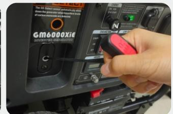
b. Electric Start: Press the engine switch upward to the Start position "Start" for 2-3 s.
