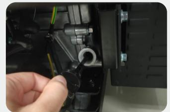
3. Place the container and tilt the machine to drain the oil;
