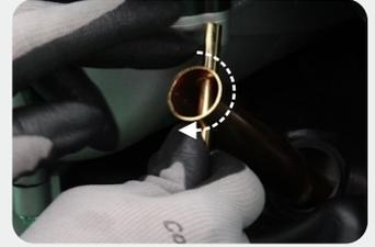
**Tip:** If there is no torque wrench when installing the spark plug, a better estimation method is to screw it 1/4-1/2 turns by force after screwing it in place, but the spark plug shall be screwed to specified torque as soon as possible.
