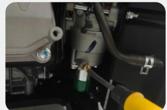
6. Allow fuel to drain into the container and tighten the drain screws on the carburetor.
