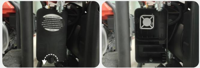
2. Clean foam cleaner element with cleaning solvent and blow it dry, Put a few drops of oil on the filter element;
