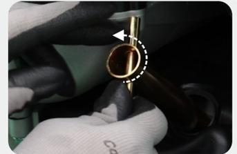
3. Check whether there is discoloration, and remove carbon deposits. Check whether there is little pale to moderate brown on ceramic cores around center electrode of the spark plug;
