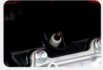
2. Insert the screwdriver into the sleeve, to screw it counterclockwise, and then remove the spark plug;
