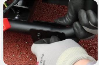
2. Fasten the nut to the bolt, tighten with a wrench. Install the other side in the same way.
