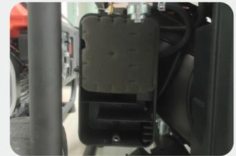
4. Reassemble empty air cleaner cap back to original position, and tighten screws.
