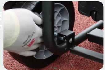
2. Insert the R pin into the hole in the wheel shaft. Install the other side in the same way.
