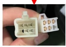
Stepper motor socket (female socket)
