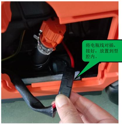
Insert the battery wire pair and place it back to the mold
