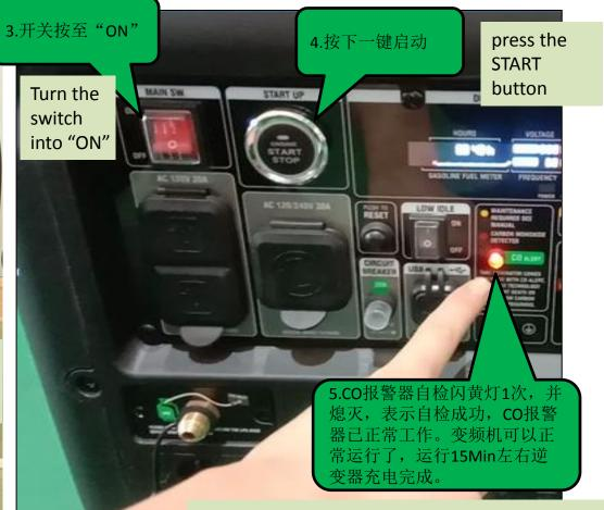
CO alarm self-checking yellow light flashes once, it shows self-checking works. CO alarm can works normally. Generator can work normally, and the generator battery is charged after running for about 15 minutes.
