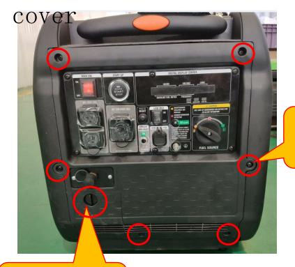
10. Assemble the panel rear cover in place and assemble the 6 Phillips
