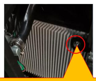
8. Install the inverter in place and align it with the through holes of the bracket. The two positioning columns of the bottom plate are installed in the bottom plate.
