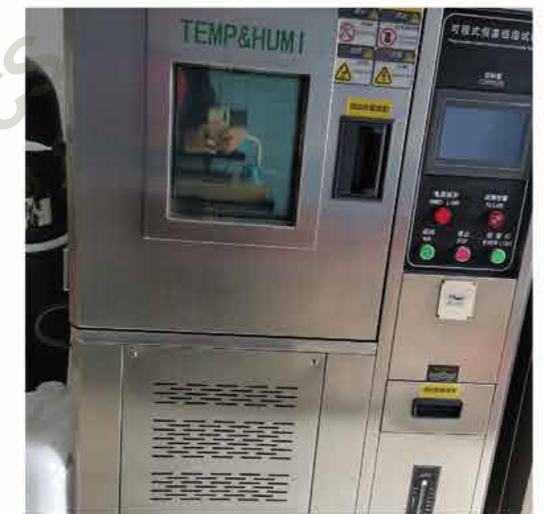
Constant Temperature and Humidity Test Chamber
